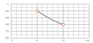
Please observe cure parameters closely since mechanical properties will develop before full cross-linking!
