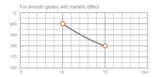
Please observe cure parameters closely since mechanical properties will develop before full cross-linking!
