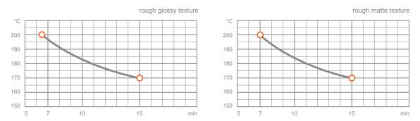
Please observe cure parameters closely since mechanical properties will develop before full cross-linking! To obtain optimal stoving conditions you are recommended to carry out practical trials each time, adapted to the carry out practical trials each time, adapted to the object in question and the stoving oven. Temperature conditions of curing for each powder listed on the label. **Our technical service department will be glad to advise you**.
